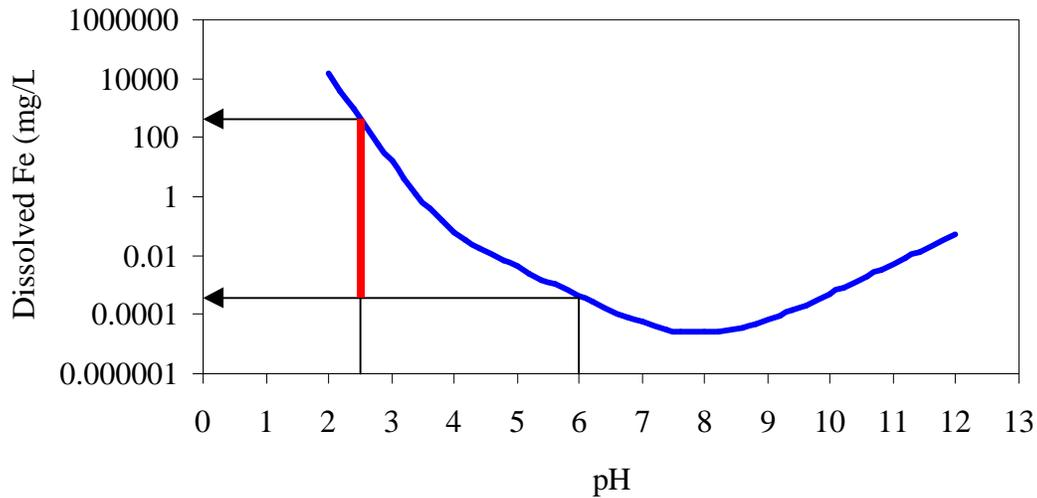
Figure 2. Overall dissolved iron solubility as a function of pH for a solution containing 500 ppm  $\text{SO}_4$ . Assuming an initial pH of 2.5 and a desired final pH of 6.0, the thick vertical line represents the mass of iron that must be removed by precipitation. Equilibrium constants from Lindsay (1979).
