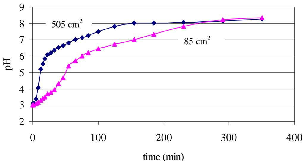
Figure 3. Effect of limestone surface area on the complete neutralization of an acid solution without iron. Both systems have the same mass of limestone, initial pH and final pH, but the rate at which they reach that final pH is faster for the system containing the larger limestone surface area. This figure differs from Figure 1 in that both systems have the same mass of limestone.
