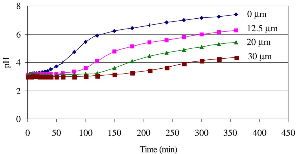
Figure 5. Effect of the thickness of the iron oxide coating on the neutralization of 0.100 mM Fe solution. Increasing the thickness of the armor decreases the neutralization rate and increase the time required to reach some final pH.
