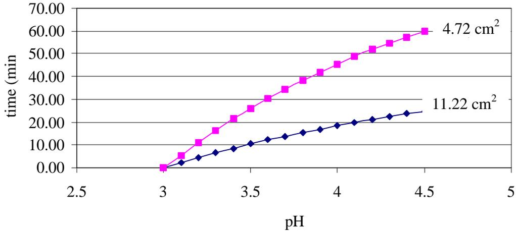
Figure 1. The neutralization rate of acid solutions containing two different-sized limestone particles. Decreasing the total surface area of limestone in contact with the solution increases the amount of time required to reach a given pH.
