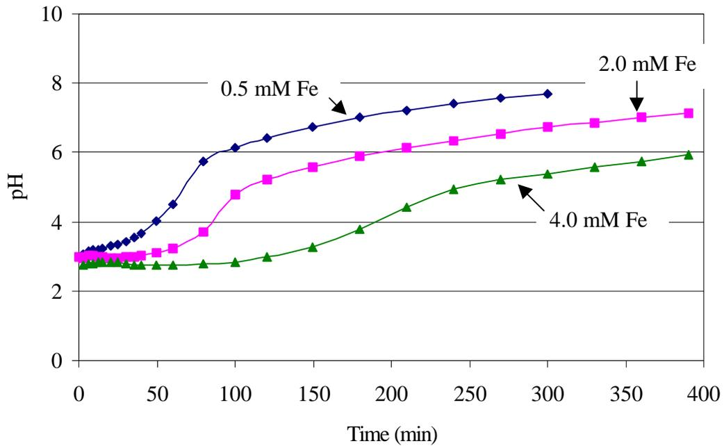
Figure 4. Effect of iron concentration on the neutralization rate of acid solutions by limestone. Increasing the iron concentration increases the lag time before neutralization begins and increases the total amount of time required to reach some final pH.
