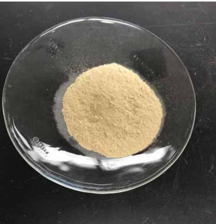
*Figure 4. West Virginia University's REE Extraction Facility produces highly concentrated rare earth products from AMD precipitates. This sample is 87 percent rare earth oxide.*
